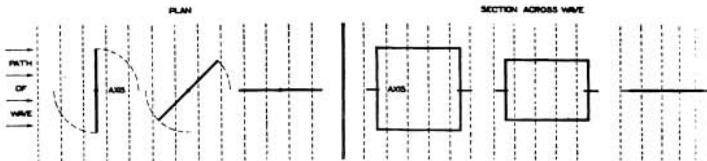
Fig. 5. Results obtained when frame is rotated on an axis not vertical. Lines of E force (shown dotted) vertical. Frame on horizontal axis. No response at any angle, the frame axis being at right angles to the path of the wave and to its lines of E force.
